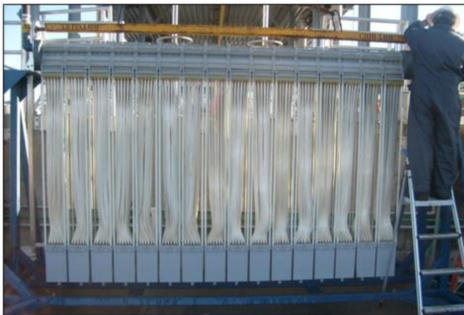
Figure 2 A typical MBR Rack Assembly fitted with sixteen MEMCOR® B40N Membrane Filtration Modules. It is mounted on a Rack Maintenance Stand and has a Rack Spreader Bar (Lifting Beam) attached to the Lifting Plates at each end.
