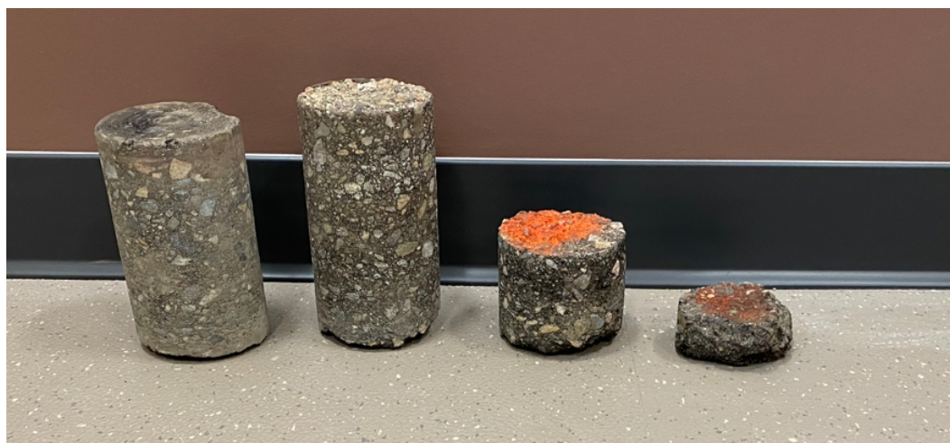
Picture of Core Samples. Left to right – Block Cracking section near 2 nd Ave, block cracking section 200’ north of Bohn Ct, fatigue cracking section near southernmost school crosswalk, fatigue cracking section near northernmost school crosswalk (bottom 2” of this core disintegrated)
